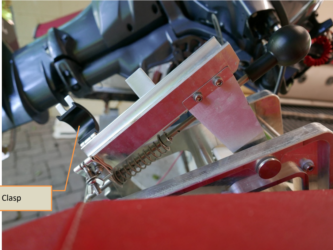
Figure 21. ReefScan Bracket – Mount for the Survey Unit showing the lower clasp.
