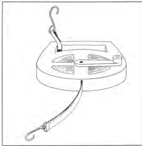
Figure 2.20 Hooks attached to the tape and casing help secure the tape during surveys.
