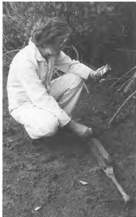
Figure 3.5 Taking readings from a core sample collected using a D-corer.
