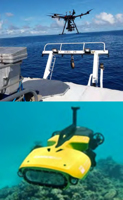
Figure 2. Platforms deployed to capture the target reef dataset (L to R) AIMS Hyperspectral Drone; QUT's WAM-V equipped with AIMS' sonar and imaging payload (on-platform and towed); Rangerbot Autonomous Underwater Vehicle (AUV). Images: Top Left, Jon Kok; Bottom Left, QUT; Right, Geoff Page.
